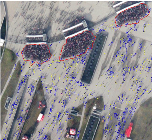
Figure 6: Results of the tracked people (yellow) and the reference data (blue), the tracks are pruned to the last six frames. The detected dense crowds are shown with red boundaries.
