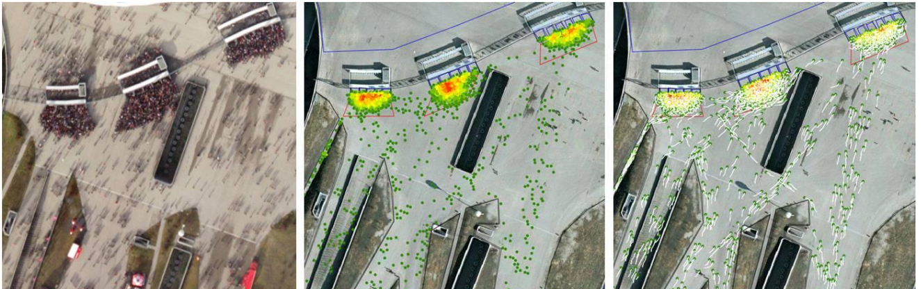
Figure 5: From left to right: Real-world data, actual position simulated pedestrians, moving direction of simulated pedestrians as snapshots at the end of the sequence.
